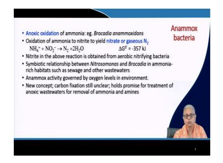
Then we come to anammox. What is anammox? Anammox is a very interesting way of oxidising ammonia in the absence of oxygen. So, in nitrification, we are utilising oxygen, but in this case, what happens is that organic nitrogen has been converted to ammonium form. And this ammonium, along with nitrite will result in the formation of inert nitrogen gas along with water.
