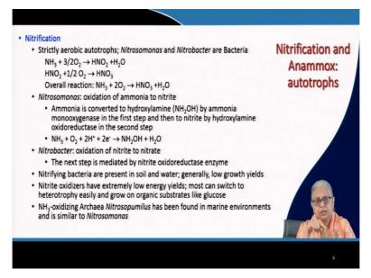
Now, this ammonia conversion to nitrite  $NO_2^-$  and nitrate  $NO_3^-$  is mediated by *Nitrosomonas* and *Nitrobacter*. So, these are specific species of aerobic autotrophic bacteria that are responsible for oxidising ammonia  $NH_3$  to  $NO_2^-$  and  $NO_3^-$ . And the first step; *Nitrosomonas* is the species that will oxidise ammonia to nitrite. In this case, this 1-step process which we generally talk about as ammonia to nitrite is actually a 2-step process.
