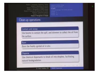
Now, how do we perform this clean-up operation? So, there are three methods one is contain and scoop. So, in this method we use booms to contain the spill and a skimmer to collect the oil from the surface.
