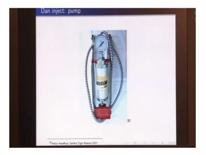
Now, in place of using a pressurized gas canister, we can also make use of these pumps now this is a pump that can be used by pressing of a foot. So, in that case also we can select the pressure that needs to be given and then this pump can be used in the field situations.
