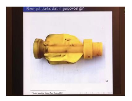
And then when this dart is fired this is what will happen because, these parts are made out of plastic. So, in the case of the explosion this plastic may get burnt, it may get walked, it may get wobbled and in that case the flight path of the projectile will be have hazard and this dart will not be able to work properly.
