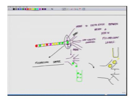
Now, I have a sensor say for example, I allow the cells to flow. So, I have something like this a very narrow tube through which only one cell at a time can flow. And here I have a sensor and here I have a gate.
