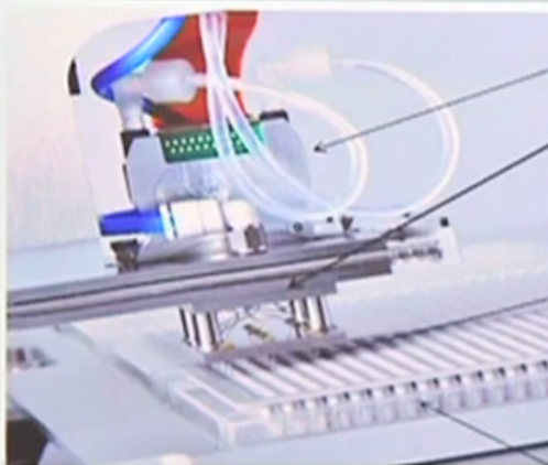
JetSpyder simultaneously addresses 12 or 32 samples
