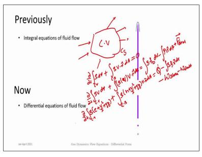
There are really two kinds of approaches looking at analyzing fluid flows. In the control volume approach or the integral forms we are really looking at analyzing the fluid flow through a certain system which is a control volume. And we look at how changes happen within the control volume due to fluxes which happen across the control surfaces. So you have control surfaces and control volume and we write the mass momentum and energy balance in an integral form.
