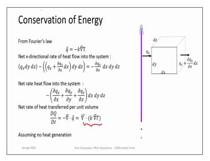
Now we have to relate how heat gets into the system how work is getting done on the system. So heat coming into the system is getting transferred by conduction is Fourier's law of conduction  $-k\vec{\nabla}T$  and you have to consider different surfaces how heat gets transferred the net rate of flow into the system is nothing but gradient of this  $k\vec{\nabla}T$  which is  $\vec{\nabla} \cdot k\vec{\nabla}T$ .
