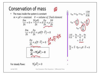
So you should just revise them if you haven't if you need to again so if you consider a very, very small fluid parcel a very small fluid element. And we are going to do analysis on such a small fluid element which is infinitesimally small. The mass inside that particular element is nothing but  $\rho v$ . So what we should say is that mass is constant, mass does not change so  $\frac{Dm}{Dt} = 0$ .
