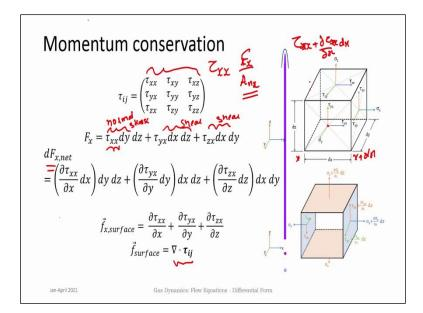
If you take any small volume it has let us take this Cuboidal volume it has different surfaces. And at each surface you will have forces that occur both in the same directions. For example if this is the x direction then you have forces along x direction and you have forces along y direction as well as this direction at a particular point. So if you take any particular point and have different surfaces you have forces along different directions.
