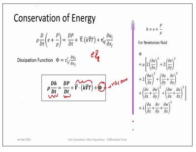
And therefore this pressure term comes within the brackets  $\left(e + \frac{P}{\rho}\right)$  is nothing but enthalpy, *h*. So finally from the conservation energy conservation term we get the equation for change in enthalpy  $\rho\left(\frac{Dh}{Dt}\right)$  is equal to changes in pressure  $\frac{DP}{Dt} + \vec{\nabla} \cdot (K\vec{\nabla}T) + \Phi$  this is the conduction heat transfer and viscous dissipation term. So,  $\Phi$ , this is viscous dissipation. This is first law
