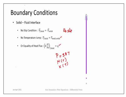
Along with you have to apply relevant boundary conditions the appropriate boundary condition is that at the fluid solid interface the velocities of fluid and solid are the same which is no slip condition. And temperature you can when looking at the temperature boundary condition you can either be that the temperature at the fluid and solid are the same no temperature jump across them.
