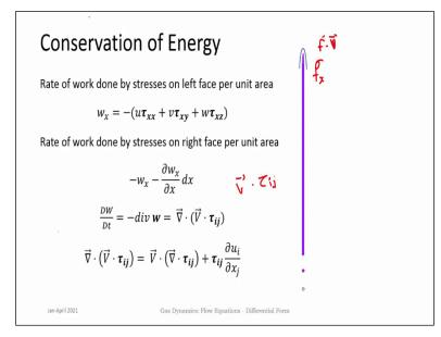
Now; what about work done in a similar manner as before we will be considered heat transfer we are checking the work done. And work done you knows the force multiplied by velocity or if  $\vec{f} \cdot \vec{V}$  is the work done. So if you take  $f_x$  the force, force in x direction it has components
