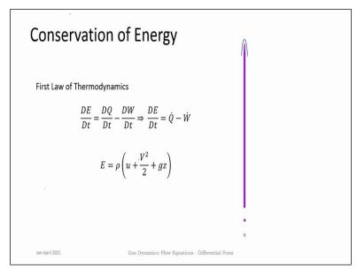
Now if you consider the energy conservation it comes back to first law of thermodynamics change in energy is related to heat added and work done on the system. So here it is given negative sign so it is a work done by the system so  $\frac{DQ}{Dt} - \frac{DW}{Dt}$  energy is composed of internal energy, kinetic energy and potential energy. So total energy is  $\rho$  multiplied by this particular thing.
