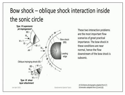
Now if we move to the interaction Shock-Shock interaction with which is very close to the sonic circle within the sonic circle? What happens here in this region 3 and region 4 they are called type 3 and type 4. Here the Bow shock is of very high strength, strength is larger flow downstream of the Bow shock is subsonic. So, that is quite different from the cases in type 1 type 2 or type 5, type 6 which had supersonic flows downstream.
