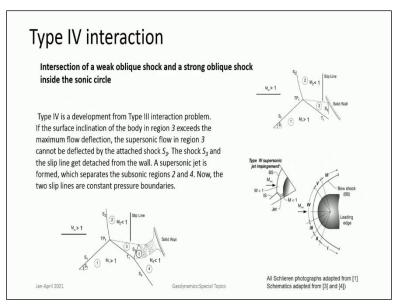
Now we can go to the most special case which is the type 4 interaction. In type 4 interaction the interaction happens very close to the stagnation region. So, much stronger shocks and if we compare it with type 3 in type 3 there is a shear layer or slip line which comes and interacts with the wall and to turn the flow that is turn the flow parallel to the wall a shock  $S_3$  develops.
