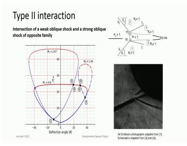
So, if we try to draw a shock polar for such interactions, we see it is possible to do that and here you find that this shock polar which is for Mach number 1.44 corresponding to a type 2 interaction does not have a solution where it intersects with any of the other shock polar but only at along the main shock polar. So, which is at this point, so, you have the 2 points here 3, 5 and 4, 6.
