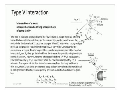
So, but these are relatively weak interactions type 6. Then we come to type 5 interaction in a type 5 interaction is. So, just like there was a distinction between type 1 and type 2 as the strength of shock increased. Similarly in type 5 here the strength of shock has increased compared to type 6 therefore again here you get a shock  $S_5$  in between and this for creates a zone which is bounded by 2 slip lines and there is a supersonic flow.
