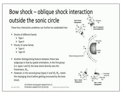
So, first let us just look at shock interactions happening with weak shocks away from the sonic circle beyond the sonic circle the flow is their shocks are relatively weak type 1 is a relatively weak shock. So, they are called as type 1, type 2, type 3, type 4, type 5, and type 6. In type 3 and 4 the shock interacts within the sonic circle where flow is subsonic after that.
