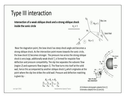
Let us consider the type 3 interaction in type 3 interaction this is the impinging shock  $S_1$  this is the Bow shock  $S_2$  and here a slip line is formed between 2 regions which is first region 2 which is downstream of a strong shock. So, subsonic flow here  $M_2 < 1$ , but region 3 which is downstream of an Oblique shock. So, in region 3 Mach number is greater than 1 a slip line is formed which intersects the solid wall.
