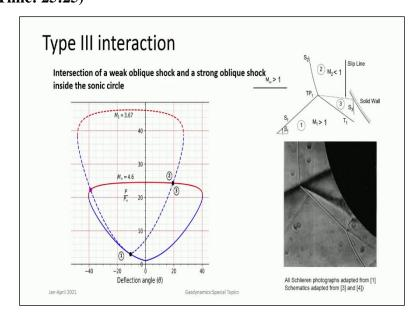
So, this is the flow picture for Schlieren of such an image. So, here you can see these are the shocks and here you have the slip line originating over here and impinging on the body around this region. The corresponding shock polar it is drawn for the triple point  $TP_1$  and 0.213 are located here.
