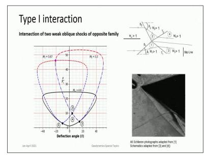
Then draw simple shock polar for this we can find out the base shock these are scaled shock polar plotted in actual coordinates. And this black line represents the upstream flow which is having Mach number of 4.6. The 2 shocks they are represented by this shock polar. So, you can see here this is one kind of a shock while the other one is in the opposite kind and they both intersect at this point which is 3, 4.
