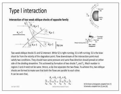
So, let us look at sharks first we look at type 1 interaction, here 2 shocks interact of opposite kind. So, this is a left running shock  $S_1$ , while  $S_2$  is a right running shock, both shocks are relatively weak. So, consequently there are 2 other shocks that are formed  $T_1$  and  $T_2$  over here now the way to analyse them is to consider different Oblique shocks this is region in 0 or you can consider the free stream.
