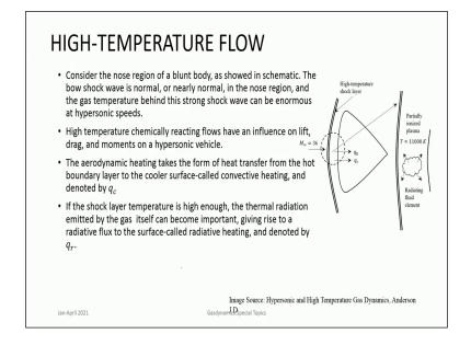
As has been now sort of mentioned often the Hypersonic flow is a flow where temperatures become very high due to conversion of kinetic energy to the internal energy of the gas. So, when temperatures become very high then the nature of the gas itself can change. So, when temperatures are as high as 11000 K taken by considering a calorically perfect gas it can be bizarre numbers like 11000 K or 20000 K and so on.
