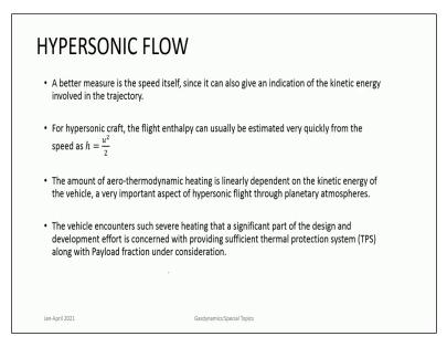
Mach number in general, it relates how the kinetic energy of the flow is related to the internal energy of the flow itself. So, as Mach numbers increase very quickly, we find that the kinetic energy contained in the flow can be as high as the enthalpy of the flow itself. Now in that case if such a flow which has very high kinetic energy been made to slow down, which happens when a body enters atmosphere, at very high Mach numbers.
