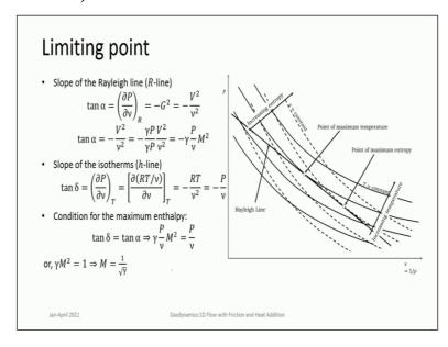
Now how do we get to these limiting points? So, this is what was meant. So, if you look at the Pv diagram these straight lines this particular straight line is the Rayleigh line. Now if you look at the curves at which h = constant. This is static points of sort of constant entropy S =constant and points at which temperature is constant that is enthalpy is constant.
