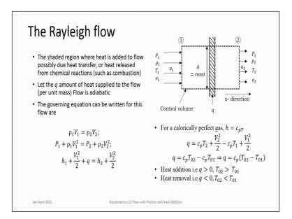
So, what are we looking at in this case this is the Rayleigh flow. And in Rayleigh flow we are looking at heat transfer or heat addition to the flow as the flow occurs in a constant area duct. Now the heat addition or it can be even heat removal. It is a non adiabatic process. So, that means heat can be transferred that can happen both heat addition or heat removal can happen.
