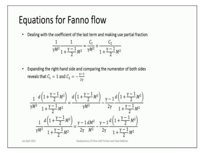
And to get the close form solution we have to express this term  $\frac{1}{\gamma M^2} \frac{d(1+\frac{y-1}{2}M^2)}{1+\frac{y-1}{2}M^2}$  terms in terms of partial fractions. And you can do that do the partial fraction expansion of this particular these particular terms plug them in the main equation.
