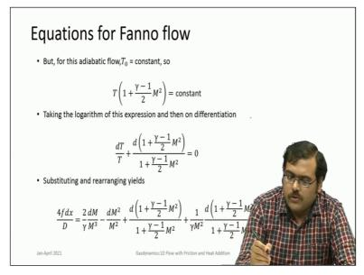
Now  $\frac{dT}{T}$  can be expressed in terms of Mach number only because in this flow T<sub>0</sub> is constant, T<sub>0</sub> = T(1+  $\frac{\gamma-1}{2} M^2$ ) This is a constant. Now  $\frac{dT}{T}$  again you can take a logarithmic differentiation  $\frac{dT}{T}$  can be
