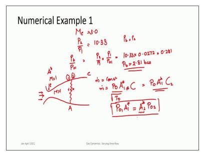
So, here the nozzle operates. So, that within the nozzle divergent portion of the nozzle you have complete supersonic flow. So, M = 3.0 but right at the exit there is a normal shock normal shock is a discontinuity. So, you have to calculate normal shock at 3.0 and pressure ratio across the normal shock  $\frac{P_2}{P_1}$  is 10.33. So, if one were to calculate what would be the exit back pressure.
