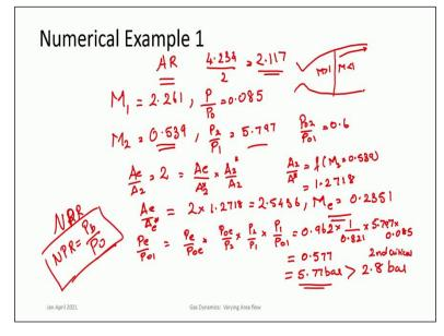
So, with this particular problem the area ratio at which the shock stance is given its half that of the exit area ratio. So, it is 4.234 divided by 2 which is 2.117. So, we know the area ratio at this point and the flow is supersonic until this particular area ratio. So, that means at the throat it was 1 and till 2.117 the area ratio of 117 it is supersonic. So, we can calculate what was the Mach number at that particular area ratio?
