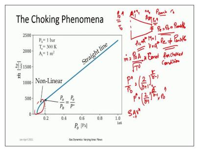
But what about absolute mass flow rate when you consider the case that the; convergent nozzle is there. Ambient pressure is held constant the ambient pressure is held constant and  $P_0$  is kept on increasing. So if you consider this case as this particular case then as  $P_0$  increases initially you have the mass flow rate increasing in a non-linear fashion. But once Mach number 1 is achieved that is Mach number becomes equal  $\frac{P_0}{P_t}$  becomes equal to  $\frac{P_0}{P^*}$ .
