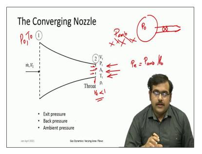
It is an isentropic flow but when the flow exhausts to certain ambient or back pressure then how does the flow behave? So these terminologies one has to understand so we are looking at convergent nozzles. So, converging nozzle or convergent nozzle, when we talk about a converging nozzle, you should understand by now that incoming flow is subsonic small velocities. And nozzle increases the flow so it increases to larger velocities.
