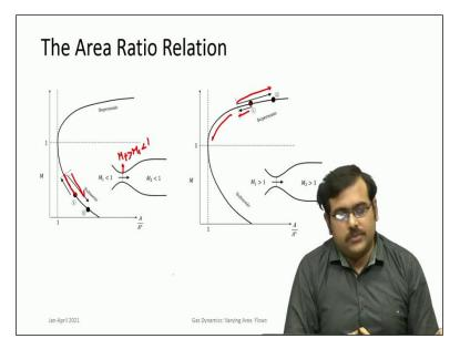
So it is not always necessary that at the minimum area Mach number should go to 1. If you are moving from a if during the motion through the convergent divergent varying area duct the flow passes from a subsonic region to a supersonic region then it has to go through a Mach number equal to 1 at minimum area. This is for a completely shock free flow when shocks are present things change a little bit.
