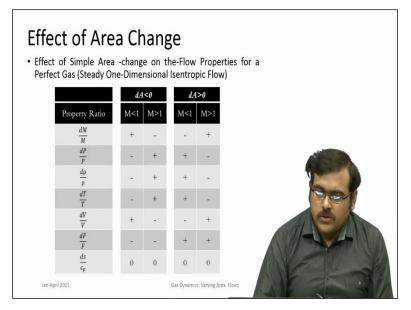
So how are they affected by area change? So, if you look at that this is for a perfect gas calorically perfect gas dA < 0 that means convergent duct. But then the flow behaviour changes between subsonic and supersonic flows. So, if the flow is subsonic then Mach number increases, pressure decreases, density decreases, temperature decreases, velocity increases the impulse function decreases there is no change in entropy.
