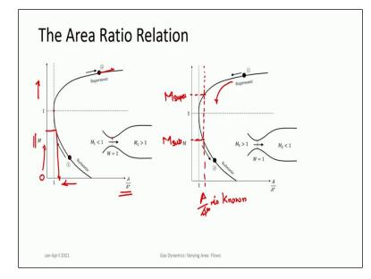
But easier way is let us just plotting it. So if you plot  $\frac{A}{A^*}$ , so  $\frac{A}{A^*}$  is here versus Mach number. So here it is plotted M versus  $\frac{A}{A^*}$  then you will find that as Mach number increases from subsonic flow. So this is 0 this is from very low Mach numbers it is going up to Mach 1 area ratio that is  $\frac{A}{A^*}$  that is often refers to as star area ratio or the area ratio sometimes used just like area ratio. So, area ratio decreases.
