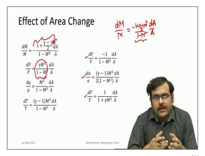
So you can do this use Cramer's rule solve the equations and you can get  $\frac{dM}{M}$  as a function of only Mach number. So as a function of only  $\frac{dA}{A}$ ,  $\frac{dA}{A}$  is the forcing gamma and Mach number. So like this we can write for all the parameters  $\frac{dM}{M}$ ,  $\frac{dP}{P}$ ,  $\frac{d\rho}{\rho}$ ,  $\frac{dT}{T}$  change in velocity, change in speed of sound, change in impulse function.
