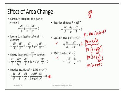
Now let us look at the sum total of all the things in a varying area duct. There is changes in velocity there is change in pressure temperature density. So, we can look at all the equations together and with  $\frac{dA}{A}$  basically the area change as a forcing function it is like a forcing. You are changing area and you want to know what happens to all these quantities. Pressure, temperature, velocity, Mach number and another parameter is the impulse equation.
