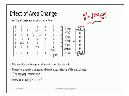
And collect all the equations together and write it in a matrix form with  $\frac{dA}{A}$  as a forcing function. Then we will know how each quantity is getting affected by  $\frac{dA}{A}$ . So this is nothing but you are expressing all the equations that have written over here for various quantities in terms of a matrix. And then this can be solved this matrix can be solved you can express  $\frac{dP}{P}$  solely as a function of Mach number, gamma and  $\frac{dA}{A}$ .
