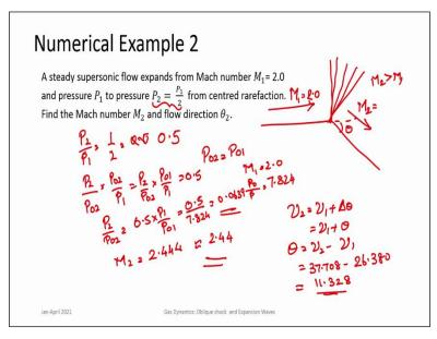
Now let us look at the next numerical example, a steady supersonic flow expands from Mach number  $M_1 = 2.0$  and pressure  $P_1$  to pressure  $P_2 = P1/2$ . So, there is it is an Expansion fan and whenever there is an expand flow passes through an Expansion fan pressure decreases. So that is evident here  $P_2 = P1/2$  from centred refraction. So, you have a centred Expansion fan you have all these various expansion fans.
