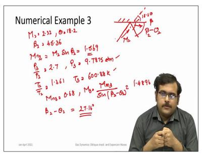
From region 2 to region 3 when we go so, we have let us remember diagram. So, the shock is coming here, and the flow is deflected, and it meets this wall the deflected flow meets the wall and another shock is formed such that after the shock the flow turns parallel to the wall. So, the flow angle that it turns by is the same as it got deflected that is 18.2°. So, this is the reference line now this is theta while this angle is beta.
