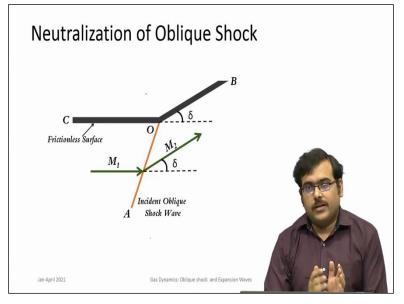
So, this is some interesting non-linear behaviour. Also, so Oblique shocks are quite different from the other waves if you can give to the wall a certain angle such that it matches the angle that the Oblique shock turns the flow with. So, it turns the flow by angle delta and at this point of intersection with the wall. The wall is also turned by angle delta. Now there is no requirement for the flow to do any further turn.
