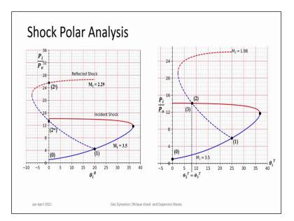
So largely what people do is look at Shock polar, now this Shock polar can be drawn for each region. So, because the Shock polar is a plot of all possible Shock waves. You can look at the Shock polar and try to find the solutions. So, the incident Shock so given a particular incident Mach number and an incident Shock you have all possible Shock waves for that Mach number is given here.
