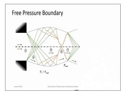
The vice versa holds good Expansion waves when they interact with the free pressure boundary, they lead to formation of compression waves which can coalesce together to form a Shock. So, like waves when like waves interact a Shock interacts with solid wall it reflects as a Shock wave. When it interacts with the free pressure boundary it reflects as an expansion wave it changes its character.
