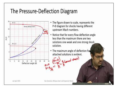
Before we go into reflection itself, it is useful to look at what are known as Pressure-Deflection diagrams. They are a plot of all possible Shock waves; Oblique shock waves also includes the Normal shock, a special case of an Oblique shock. So, if you plot all possible Shock states for a particular Mach number the pressure ratio across the Shock versus the deflection angle for one given.
