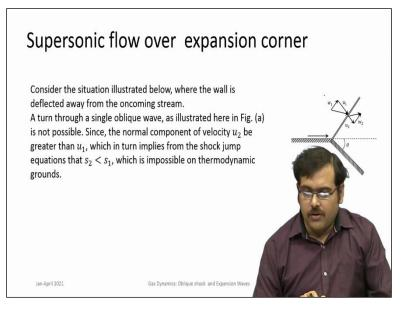
Always the flow turns away from the flow, that always happens by means of a gradual turn. So, a sharp discontinuity of this sense is not possible, that is an Expansion shock is not possible because always you should have positive change in entropy.
