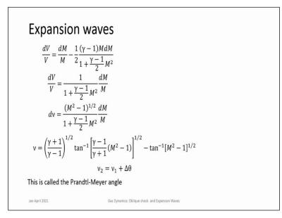
You get the M/(M-1/2) and then do the algebraic manipulations you get dV/ V is  $(1 + \frac{\gamma-1}{2}M^2)\frac{dM}{M}$  and this is substituted and so you get expression for the Prandtl-Meyer function explicitly in terms of gamma and M this is a calorically perfect gas gamma is constant this can be integrated, and this is the integration for. So, this is the Prandtl-Meyer angle.
