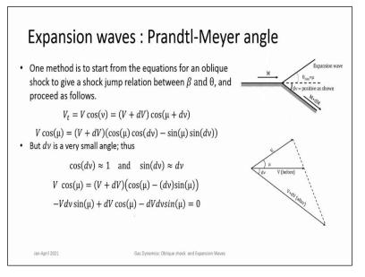
So that is this kind of an analysis is done by Prandtl and Meyer, so this is known as Prandtl-Meyer function or Prandtl-Meyer angle. How do we do this analysis? So, we again draw the velocity triangles across one single expansion wave across a wave very similar to the analysis that was done earlier for the Oblique shock. We look at the components of these velocities.
