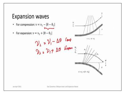
During a turn, a gradual turn so, a compression turns the Prandtl-Meyer angle decreases. So, it takes a negative sign minus delta theta. So, you should always remember these. So, for gradual turns for both compression and expansion you can use the Prandtl-Meyer analysis and you can relate the downstream and upstream conditions. So, the relationship is  $v_2 = v_1 - \Delta\theta$  for compression and  $v_2 = v_1 + \Delta\theta$  for expansion. Expansion or turn away from.
