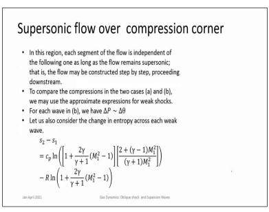
So, across each small turn there is an incremental change in pressure. So that is how it happens. There is a entropy change across the Oblique shock and the entropy change is the same as that for a Normal shock for normal component. So, that is what is written over here  $\Delta s$  for the Oblique shock, and this is for a Normal shock and here if you substitute instead our M<sub>1</sub> you substitute M<sub>n1</sub> then you get it for an Oblique shock.
