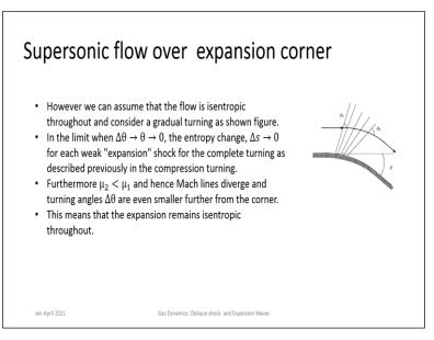
So, what is possible is a gradual turn or gradual change in flow. This is gradual turn away from the flow and the flow remains isentropic and it is bound by Mach waves. Now these are Mach waves. So, this is starting Mach wave  $v_1$  this is at the end  $v_2$  and since they are related v is
