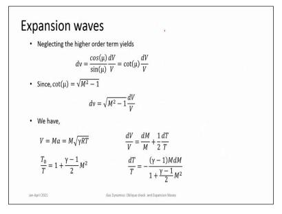
So, if you then write down this equation what you get is d nu is equal to  $\cot \mu (dV/V)$ . So, this is the equation. So, what is  $\cot \mu$ ? You can draw the angles, so this is what is  $\mu$ ,  $\mu$  is  $\frac{1}{\sin(\frac{1}{M})}$ . So, this side is  $M^2 - 1$ , so  $\cot \mu$  is  $\sqrt{M^2 - 1}$ . So that is given here. So now this expression relates  $d\nu$ , which is known as nu is the Prandtl-Meyer function to the change in velocity dV/V.
