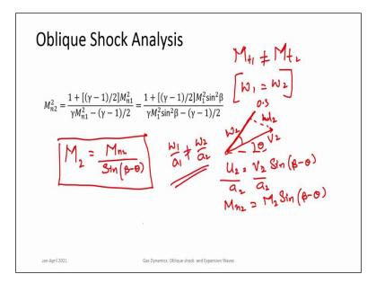
So, you can find  $M_{n2}$  which is the normal shock, the flow downstream of the normal shock but  $M_{n2}$  is only the normal component of the downstream velocity. There is a tangential component also. So, the tangential component  $w_1$  is same as  $w_2$ . Now be very careful here because the velocity triangle or the velocity diagram for this is the Oblique shock; we are looking at the downstream flow it has been turned by an angle  $\theta$ .
