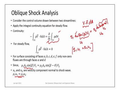
We always start with the Continuity equation, steady flow. Continuity equation in the steady flow, there is no change in the mass of the control volume. So, it is '0' and only we are looking at the fluxes across the control volume. So, it is bound between 2 streamlines so there is no flux of mass across lateral directions. So, there is no flux, so there it is a streamline and only flux that goes in is entering through 'a' and leaving through 'd'.
