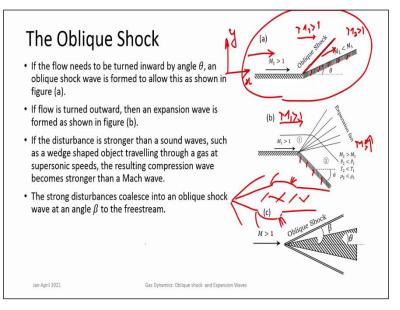
So, when are oblique shocks formed? Whenever the flow must take a turn, for example, as depicted in this schematic over here. You have an oncoming flow which is supersonic, always you should remember the Shock waves are found in supersonic flows. So, a supersonic flow is coming and then it faces a turn. There is a turn which turns the flow towards into itself or towards itself.
