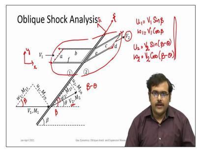
So how do we analyse oblique shock? So oblique shock analysis borrows things from Normal shocks as well as from the idea, that you had when doing moving Normal shock that you jump on to the shock. So even in Oblique shock, it is the same thing, you do this as a stationary flow, so it is a steady flow, it is not an unsteady flow, it is a steady flow. But now you see this has 2 dimensions, the Shock is oblique, it is at an angle to the flow, it is not normal to the flow.
