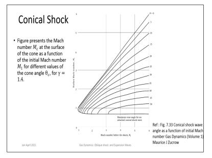
These things can be plotted, so main idea here is though you get Oblique shocks in cones also which is known as conical shock they are not the same as Oblique shocks for wedges there is a slight, there are differences. But the basic principle remains the same that if the flow must take a turn in a supersonic condition and the turn is towards itself it is a compression kind of nature then Oblique shocks are formed.
