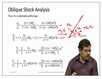
You can get all the relations for pressure ratio, density ratio, and temperature ratio. So, all of that analysis you had done for Normal shocks, you can carry on again over here and do it for the normal component of the Oblique shock. So, you have an Oblique shock here, it is at an angle  $\beta$  creating a flow deflection of  $\theta$  for an incoming flow of 'M<sub>1</sub>', Mach number M<sub>1</sub> velocity is V<sub>1</sub> and results in M<sub>2</sub>, V<sub>2</sub>.
