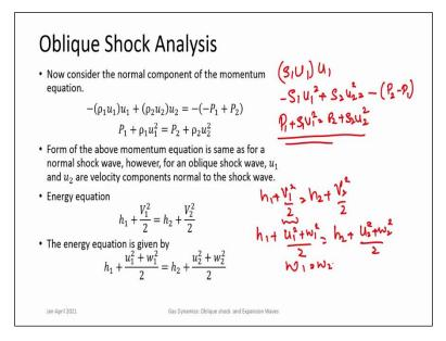
So now let us consider the normal direction. So now normal direction there is a pressure force acting which is 'P<sub>1</sub>' and 'P<sub>2</sub>' across the Oblique shock, P<sub>1</sub> before the oblique shock and P<sub>2</sub> after the Oblique shock and the momentum flux is ' $\rho_1 u_1 \times u_1$ '.
