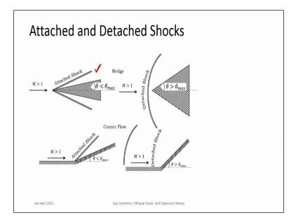
So, ending of these discussions on oblique shocks as I told initially the oblique shocks are the analysis that we did is for a 2-dimensional flow typical are plates at angles wedges and so on. The same kind of analysis can be done for cones axisymmetric bodies but there is a difference, the difference is that in the oblique shocks it is 2-dimensional. So, if you look at the streamlines, the streamlines just go across the shock and then they deflect according to the angle of the wedge across.
