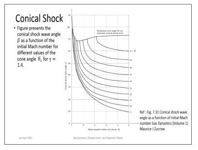
The key idea you must understand is when you are considering a conical body and shock it is the even though the shock appears oblique in nature you cannot apply the oblique shock relations there. You must use the conical shock relations these are plotted you can get these plots. One main feature you must understand is that angle of conical shock is always greater than that for an oblique shock for the same deflection angle.
