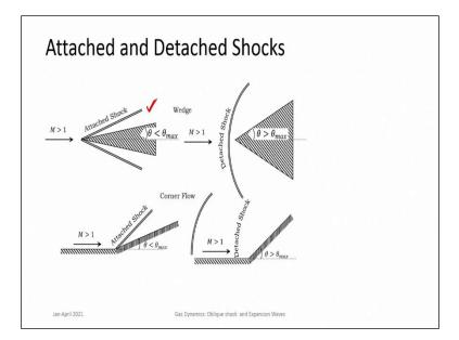
So, this kind of solution where the shock wave is attached to the wedge is called an attached solution. Here the angle of the wedge or angle of deflection is lesser than the maximum angle while if the angle is greater than maximum angle then you call it a detached shock. Then you form detached shocks like this. So, in almost all our analysis we are concerned with attached shocks but we should understand this when you do your analysis or apply things to problems.
