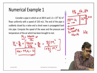
So consider this example numerical example 1. Consider a pipe in which air at 300 K and  $1.5x \ 10^3 \ \text{N/m}^2$  Pascal flows uniformly with a speed of 150 m/s. The end of the pipe is suddenly closed by a valve and a shock wave is propagated back into the pipe. Compute the speed of the wave and the pressure and temperature of the air which has been brought to rest.
