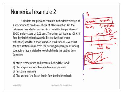
So the second example is, calculate the pressure required in the driver section of a shock tube to produce a shock Mach number 3 in the driven section which contains air at an initial temperature of 300 Kelvin and pressure of 0.01 atmosphere. So its low pressure we can draw the schematic here and here you know  $T_1 = 300$  K and  $P_1 = 0.01$  atmospheres. We do not know what is  $P_4$ . We have to find  $P_4$ . Driver gas is air at 300 Kelvin.
