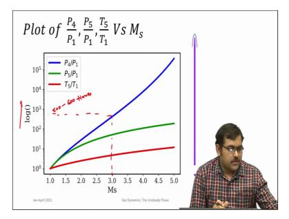
So this is a plot of  $\frac{P_4}{P_1}$ ,  $\frac{P_5}{P_1}$  and  $\frac{T_5}{T_1}$  in terms of shock Mach number this is what is desired. So, we need if you need a certain  $\frac{P_5}{P_1}$  or  $\frac{T_5}{T_1}$  then what should be the shock Mach number that needs to be given and correspondingly what should be the pressure ratio across the shock tube that needs to be given. So if you do find and calculate that you can see that the scale is in log.
