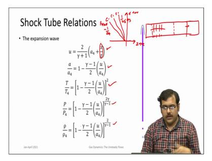
So, to put; now if you look at the entire shock tube. So you have you got the equations for shock wave you got the equations for the contact surface. Now we have the equations for the expansion fans which come here. So the velocity in the expansion fan it varies gradually that is a function of  $\frac{x}{t}$ . You have to bear in mind that the xt diagram for an expansion fan is like this.
