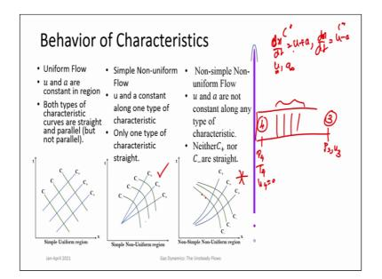
So how can we apply this to shock waves shock tube problem. To get the connection we need to understand a little bit about how these characteristics behave? So, if you have a region of uniform flow that is the velocity, pressure and temperature do not depend on space and time and there you draw the characteristics  $C^+$  and  $C^-$ . The  $C^+$  and  $C^-$  are nothing but  $\frac{dx}{dt} = u + a$  and This is  $C^+$  and  $\frac{dx}{dt} = u - a$ . This is  $C^-$ .
