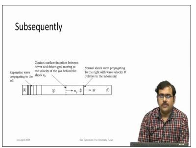
So as soon as the diaphragm ruptures there is a large pressure difference between the two sections, and it is a compressible gas in inside the tubes and so you have compressible flow
