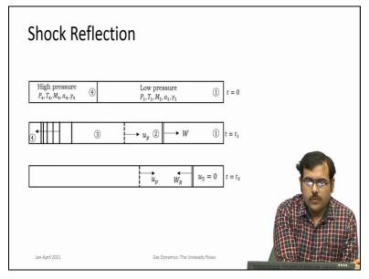
So now the shock wave can go all the way. Suppose this shock tube is closed at both the ends then the shock wave proceeds all the way towards the end of the shock tube. So at the end there is a solid wall and boundary condition there is that the flow cannot penetrate inside the solid wall. So the bulk motion of gas that was happening behind the shock with a velocity u2 on meeting the wall should abruptly stop or come to a velocity as soon as it meets the wall its velocity should become zero.
