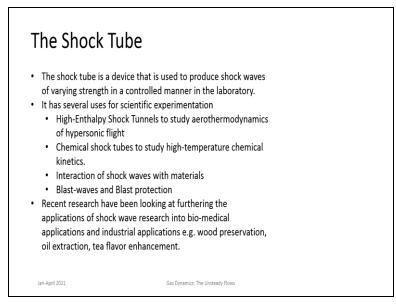
Now it is a device that is used to produce shock waves in a controlled manner and of varying strength but mostly in the laboratory and it has several uses for scientific experimentation. And mainly it is used in high enthalpy shock tunnels to study aerothermodynamic phenomenon of very high Mach number flows. We know when Mach number increases
