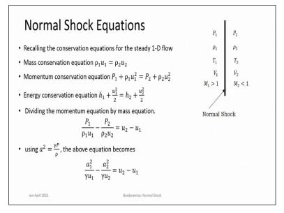
This is something that was done the previous class. So, I will quickly go through this and the conservation equation of mass, momentum, energy for one dimension is used to analyse the normal shock. It is an adiabatic process without any work done. So, you can apply these equations along with the equation of state and relation for the enthalpy.
