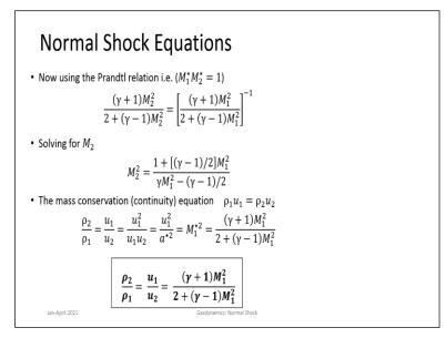
So that we can exclusively get the equation for downstream Mach number  $M_2^2$  in terms of  $M_1^2$  and  $\gamma$ . Similarly using the continuity, once we had done this, we can get the equation for the density ratio  $\frac{\rho_2}{\rho_1}$  in terms of only Mach number and  $\gamma$ . So, this is something that will come up again and again
