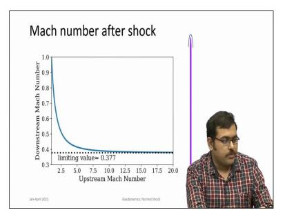
So another interesting thing about the downstream number of shock you see that always you have the Mach number downstream of the normal shock to be subsonic a normal shock exists only in supersonic flow. So upstream is supersonic downstream is subsonic the way  $M_2$  behaves is that it decreases but then similar to the way density sort of saturates by increasing to a value.
