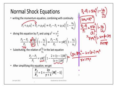
So now we are left with the pressure ratios, temperature ratios. Let us see how to get to them. So here we take the momentum equation again equation  $P_1 + \rho_1 u_1^2 = P_2 + \rho_2 u_2^2$  and do the subtraction the sort of moving the variables from here to the side is  $\rho_1 u_1^2$ . Now once we have the Prandtl's relation that is relating  $u_1 u_2 = a^{*2}$  for conditions across the normal shock.
