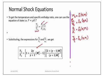
Now once you get the pressure ratio then getting temperature ratio is nothing but using the ideal gas equation of state. So  $P = \rho R T$ .  $\frac{T_2}{T_1} = \frac{P_2}{P_1} \frac{\rho_1}{\rho_2}$ . Now  $\frac{P_2}{P_1}$ , we have the expression for this,  $\frac{\rho_1}{\rho_2}$  we have the expression and so we can multiply the 2 expressions,
