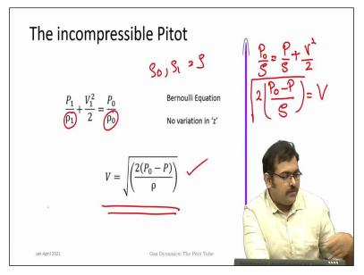
This condition must be very familiar to all, this is the incompressible Pitot equation. In this the principle used is directly the Bernoulli equation there are no losses that is the basic definition of the stagnation process. This is a incompressible flow so density remains a constant. These  $\rho_0$ , and  $\rho_1$  all of them are equal to ' $\rho$ ' and so you write the Bernoulli equation considering that there is no variation in the potential energy.
