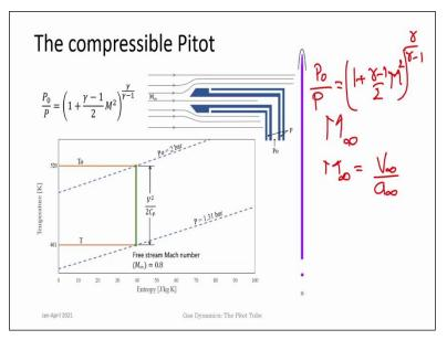
The process happening within the Pitot tube is a stagnation process, where you have the flow coming in and it stagnates within the Pitot tube. Once you measure both  $P_0$  and P then this is a compressible flow now you have Mach numbers which are greater than 0.3 then, have to use the stagnation process and under stagnation process the relationship between  $P_0$  and P for calorically perfect gas is,
