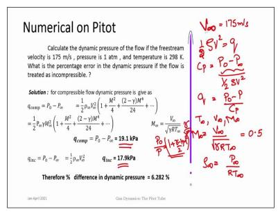
Now just let us look at briefly how these things compare so just by using a simple numerical. Calculate the dynamic pressure of the flow if the free stream velocity. As here it has been written as free stream velocity which is 175 m/sec. Pressure is 1 atm and temperature is 298 K. what is the percentage error in dynamic pressure if the flow is treated as incompressible?
