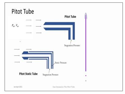
Pitot tube must be familiar to all; it is a flow measurement technique, it is simple in constructions basically a tube. Hollow tube into which the flow coming in, at any particular point if you introduce a Pitot tube then the flow that is coming into the tube goes and stagnates within the tube and the pressure within at that particular point is measured using any pressure measurement system.
