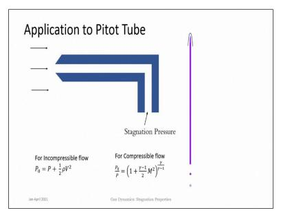
This understanding of the stagnation properties is important and this is applied directly to flow measurement through the use of Pitot tube which will be discussed in detail in the next class. (**Refer Slide Time: 31:39**)
