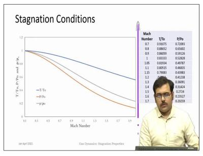
You can immediately notice that this formulation  $(1 + \frac{\gamma - 1}{2}M^2)$  for temperature ratio is fairly straight forward. But for pressure ratios and density ratios you have exponentials. While calculating, the way these principles are used is usually that you will know the velocities or Mach numbers and have to estimate the stagnation conditions.
