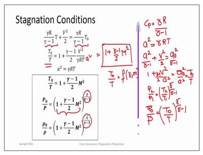
This is using the relation that  $c_p = \frac{\gamma R}{\gamma - 1}$ , gamma ( $\gamma$ ) is the ratio of specific heat for the gas and R is a specific gas constant. So once that is substituted you get these 2 equations here. And we also use the fact that  $a^2 = \gamma RT$ , where 'a' is the Speed of sound. This equation then becomes  $\frac{a^2}{\gamma - 1}$ .
