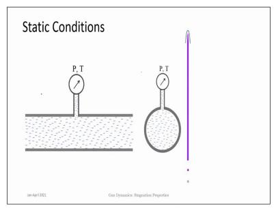
So, the common principle for both of them is the static condition and then you can reach the stagnation conditions or the sonic conditions through a certain hypothetical process. So, static conditions are the normal conditions of pressure, temperature in a fluid flow. For example, you have a fluid flowing through a duct here. At any point if you take, for example at this local
