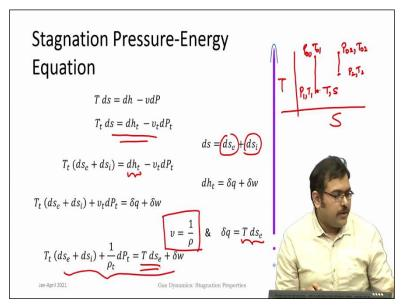
So, coming into the specific case of the stagnation pressure, now if you look at the TS diagram; you can immediately make out that for every point in a flow peak T, s or this is any particular pressure, and temperature. In a TS diagram you can always associate a stagnation condition
