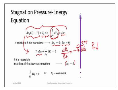
Now this is algebraically rearranged to terms containing only energy exchange process terms containing only irreversibilities, work done and the total pressure. So this equation in total is known as the stagnation pressure and energy equation. So there is stagnation pressure here and the rest of the terms relate energy and work done. Now specifically if you look at this equation and take that it is an adiabatic process. In an adiabatic process there is no heat exchange happening.
