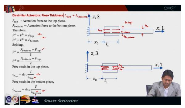
Now, all we need to do is to find out the displacements, axial displacements at this junction: the top surface of the beam and the piezoelectric patch where they are meeting, and at the bottom junction, the bottom part of the beam and the bottom piezoelectric patch where they are meeting. So, at the top surface of the beam, the extension is delta  $l_{btop}$ , which is this.
