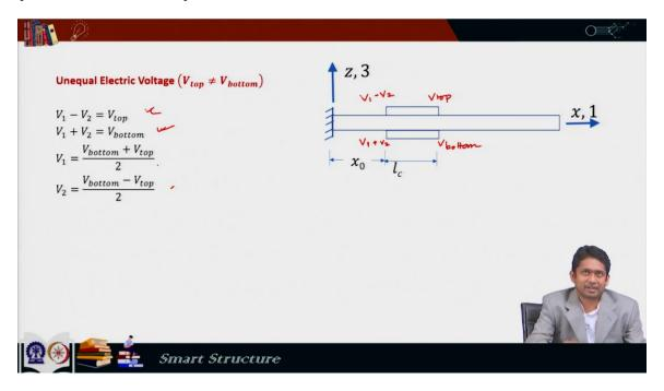
So, from whatever we did on the symmetric and anti-symmetric actuation, I mean the axial and bending actuations, we can say that the actuation force due to  $V_1$ , the extensional or axial force is  $F_{bl_1}$  multiplied by  $EA_b$  by  $EA_c$  plus  $EA_b$ .
