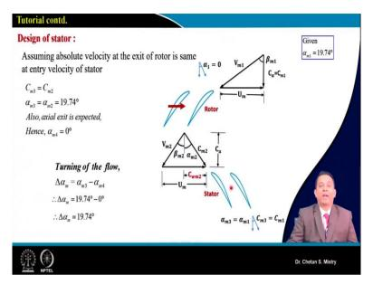
So here, this is what is a design for our stator. If we look at for the stator the assumption that's what is the flow which is coming out from the rotor that's what is coming at absolute velocity  $C_2$  and angle  $\alpha_2$  and as per our conventional design what we are doing? My  $\alpha_2$  and  $\alpha_3$ , they both are same, and since this is what is a fan in which we are considering our exit to be axial one.
