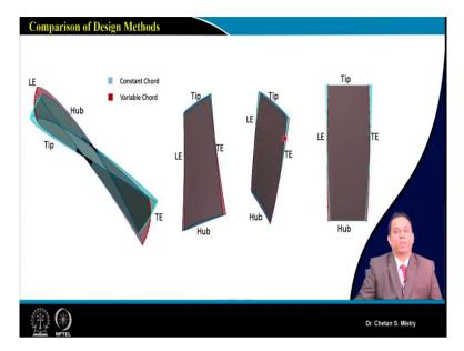
Here, this is what is with the constant chord of 450 mm we can say this is also been stake about the CG point. And, if we compare these two blades, we can easily understand how my twist of the blade, that's what will be coming with. Because we are having change of our chord, all the way from hub to tip and this is what is representing how my dimensions that's what is changing all the way from hub-to-tip, okay.
