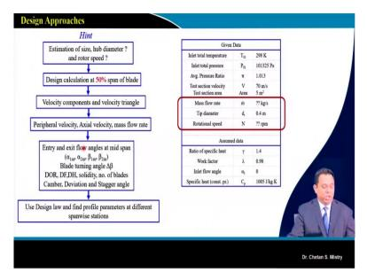
We have our inlet pressure, temperature; we know our pressure ratio, test section velocity, that's what is say 70 m/s; mass flow rate, total tip diameter, rotational speed, all those things, that's what we need to decide with. So, mainly here if you look at, this is what is our important parameter for the design of this fan. So, how do we start with is to estimate the size, we need to decide with the hub diameter, we need to decide with what will be the rotational speed, okay.
