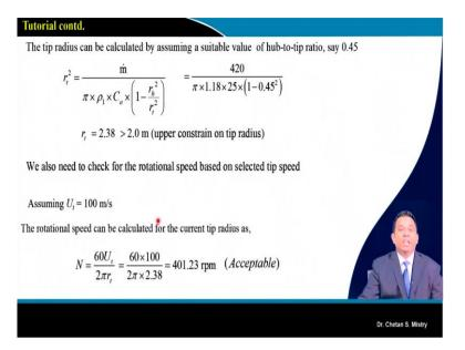
Now, with this if we are putting that in our mass flow rate equation it will give the diameter of the tip and that tip diameter it is coming 2.38 m, that's what is on higher side.
