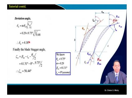
Now, deviation angle also we can calculate based on carter's rule, it is coming 4.18. We can calculate our say stagger angle; this stagger angle, it is coming 56.44°.
