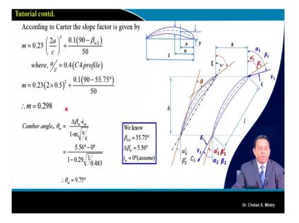
Now, once this number of blades they are being calculated, we can do calculation for say our cascade parameters. So, we will be calculating our Carter's slope factor based on our calculation of  $\beta_1$  and  $\beta_2$  that is coming 0.298.
