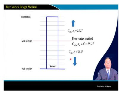
So, based on all these calculations we are able to calculate the parameters at the mid station. Now, what is our next requirement? It is to calculate the flow angles at different stations. So, what we will be doing? We will be dividing whole span into maybe 10 or 20 number of stations. Here in this case, we are dividing that into more number of stations. We know for free vortex we can calculate our  $C_w \cdot r = constant$ .
