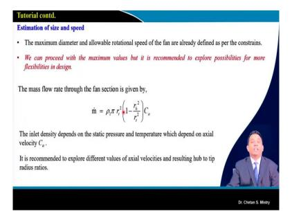
Now, next step for our design it is to decide with the size and the speed. The maximum speed that's what is defined saying like 500 RPM and maximum diameter, they both the things are known to us. So, by that way we can start doing our design, but in order to understand what all are the other possibilities because they are also equally important and that is the reason why this design it has been explored in a different way.
