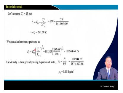
Say, initially suppose say we are assuming our axial velocity to be say 25 m/s. If we know our axial velocity, we can calculate what will be the pressure and temperature in sense of static terms. So, static temperature we can calculate it is 297.68 K and static pressure that is coming 100.94 kPa and based on that if we calculate our density, the inlet density that is coming 1.18  $kg/m^3$ .
