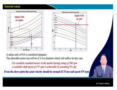
And, looking to this demand, if we go through, we can select the radius ratio roughly to be in the range of 0.6. Suppose say, I am taking this to be 0.6 this is what is giving us idea what need to be the axial velocity. At the same time, as we have discussed, we have constrain with the rotational speed of the motor. Because 750 kW motor, it is a huge power capacity and that's what will be rotating at the lower speed and that speed, that's what is a constraint up to 500 rpm.
