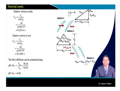
Now, based on the velocity triangle since this is what is say axial entry, we can say relative velocity at the entry is given by  $C_a/\cos\beta_1$  and this is coming 91.65 m/s.
