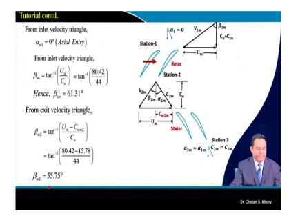
Now, once we are having mid station calculation, we know our  $\alpha$  that is 0, we can say from our inlet velocity triangle we can calculate our  $\beta$  that's what is  $\tan^{-1}(U_m/C_a)$ . My mid station peripheral speed is known we can calculate our  $\beta_1$ . We can calculate same way  $\beta_2$ . Now, this  $\beta_1$  is coming 61.31° and  $\beta_2$  is coming 55.75°.
