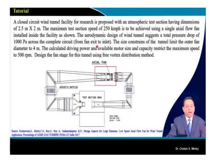
So, the details are closed circuit wind tunnel facility for the research is proposed with an atmospheric test section having dimensions of 2.5 m by 2 m. Maximum test section speed is  $250 \ km/h$  to be achieved using single axial flow fan installed inside the facility; this is what is a fan we are discussing about. The aerodynamic design of wind tunnel suggests the total pressure drop is 1000 Pa across the complete circuit.
