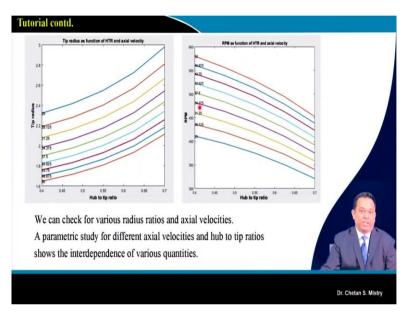
What it says? This is what is representing my hub-to-tip ratio because that's what is important parameter, when we are discussing about the fan design. Second parameter, that's what is say tip ratio and here this is what is representing different values of axial velocity. On the other side, this is what has been correlated with say hub-to-tip ratio, my rotational speed and axial velocity.
