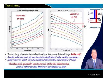
Now, what constraint we are having? We have upper constraint with the radius it says my tip radius should not exceed by 2 m, okay. At the same time, we are having constraint with the speed it says it should not be more than say 500 rpm. Now, here in this case we need to decide with what should be our hub-to-tip ratio. So, here if you look at, this is what all we have discussed earlier when I say hub-to-tip ratio of 0.8, my hub-to-tip ratio is 0.4.
