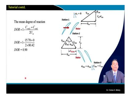
The next parameter, that is important for us is to calculate the degree of reaction, at mid station what is our whirl distribution and what is our mean peripheral speed that's what is giving degree of reaction to be in the range of 0.90.
