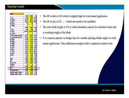
And, that's what will be helping us in sense of making this particular design sheet. So, we are having our hub station, mid station and tip station calculation. Now, once we are doing our calculation for hub, mid and tip station, it is very important to further discuss the modification and the design. So, for present lecture we are stopping here with say having calculation at mid station, having calculation at hub station and tip station.
