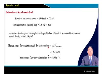
Now, in order to do so what all we are looking for is in terms of calculating certain parameters. So here, in this case what it says my required test section speed it is 250 km/h; so that's what is coming roughly 70 m/s. So, this is what is the speed we are looking for at the test section.
