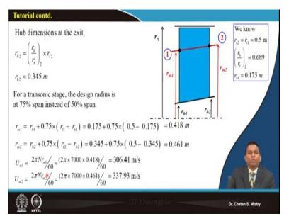
Now, here in this case, once the hub to tip ratio at the outlet station, that's what is known, we can calculate what will be the hub diameter or hub radius at the exit, and this is what is coming as say 0.345 m.
