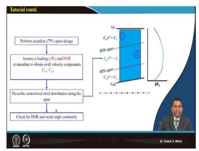
What we will be doing here? Say, in order to simplify and in order to reduce our calculation and for understanding, we will be configuring our say span of the blade into three different stations. We will be considering my first station, that's what is from hub to 40% of span then from 45 to 85% span and above 85% span.
