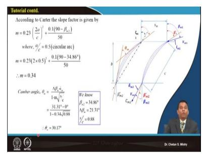
Now, we need to calculate our blade parameter or say blade airfoil or airfoil geometrical parameter that's what will be based on Carter rule. So, we will be calculating our slope factor. Here, this blade also we are considering as a circular Camber line that is why a/c is 0.5, that's what is giving me 'm' equal to 0.34. My Camber angle, that's what is coming 30.17. Here also, we are assuming our incidence angle at the mid station to be say 0.
