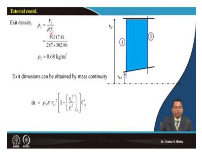
Now, once the static pressure and static temperature, they are known to us, we can calculate our static density and that's what is say  $P_2/RT_2$  that is coming as say 0.68  $kg/m^3$ .
