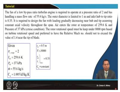
So, what we have learned from that let us try to take one of the numerical. What it says? The fan of low bypass ratio turbofan engine is required to operate at the pressure ratio of 2 and has mass handling capacity that's what is 55.6 kg/s. The outer diameter is limited to 1 m and inlet hub to tip ratio is 0.35. So, we say, these are the constraints; say we should not exceed our casing diameter beyond 1, and at the entry we are having hub to tip ratio to be 0.35.
