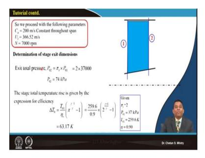
So, based on that, we can say, we are finalizing our axial velocity, that's what is 200 m/s and it is given that's what is constant throughout my span. And, our peripheral speed we are considering 366.52 m/s, rotational speed we are considering 7000 rpm. If this is what is known to us, so, at the entry condition, we can say, we are having our parameters known for making of a velocity triangle. Now, this is what is a fan that's what need to be designed, so, if we consider, this is what
