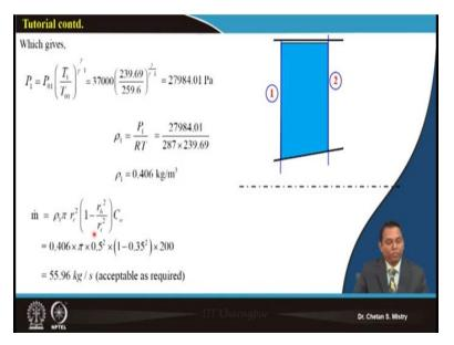
We can determine our pressure...static pressure, that's what is coming say 27.98 kPa, and we can calculate our density. This density is coming 0.406  $kg/m^3$ .
