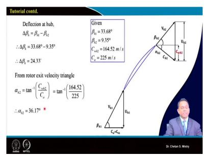
Now, here in this case, if this is the case, we can have our  $\Delta\beta$ , that's what is coming 24.33°, okay. So, with this  $\Delta\beta$ , we will be moving forward with say calculation of  $\alpha_2$ , we will be calculating what will be our relative velocities, okay. So, based on velocity triangle, we can say tan  $\alpha_2$ , that's what is  $C_{w2}/C_a$  and this is what is coming as say 36.17°.
