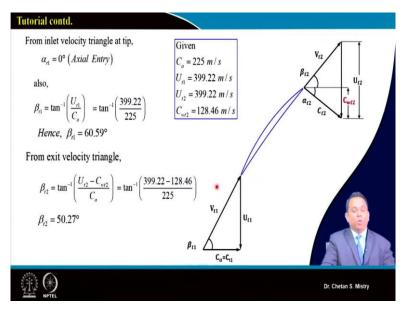
Now, based on this, we can do our calculation for different velocity components near the tip region. So,  $\alpha_1$  that's what we are assuming to be 0, we are considering axial entry throughout the span, okay. And, based on our velocity triangle we can calculate what will be our  $\beta_1$  at the tip and what will be my  $\beta_2$  at the tip. If you are considering  $\beta_1$  at the tip it is coming 60.59° and  $\beta$  at the tip, that's what is at the exit it is coming 50.27°.
