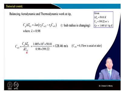
Now, in line to what all calculation we have done at mid-station and at the hub, we can do our calculation by comparing aerodynamic and thermodynamic work. So, here in this case,  $C_w$  that's what is at tip-station,  $C_{w2}$  at the tip-station, that's what we can calculate by comparing our aerodynamic and thermodynamic work. So, if you will be putting that number, it says my whirl component at tip at the exit, that's what is coming as say 128.46 *m/s*, okay.
