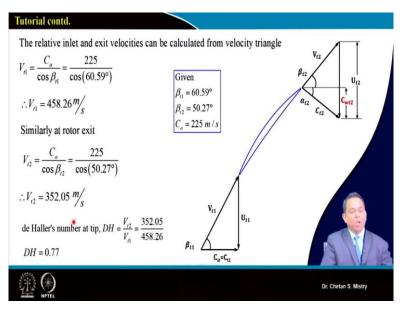
Now, based on what all calculation we have done for our blade angle, relative inflow blade angle, relative outlet angle, we can calculate what will be our relative velocity at the entry, what will be our relative velocity at the exit and based on that we can do our calculation for de-Haller's factor.
