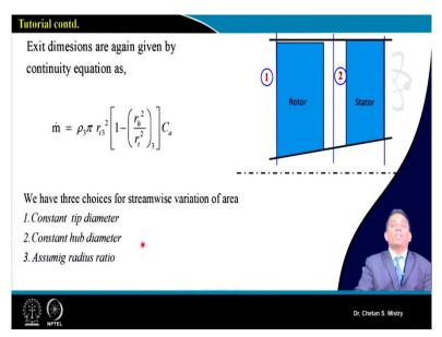
Now, if we are considering, we need to have our continuity to be satisfied both at the entry as well as at the exit station. So, when we say at the exit station, my mass flow rate equation I can write down, it is
