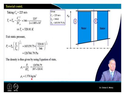
We can now do our calculation for static temperature. Now, again here in this case, we can assume our exit to be axial one. So, we can say my absolute velocity at the exit, that's what is suppose say  $C_3$ , this is equal to my axial velocity. And we are assuming our axial velocity to be constant for this configuration. So, if we are putting that as a number, it says we will be calculating our static temperature at the exit or at the station 3. So, this station 3 it is coming as say 320.81 K.
