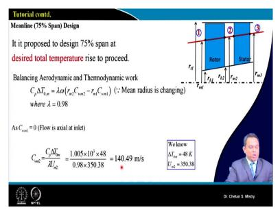
So, what it says? Now, at 75% span, we are assuming our pressure ratio to be 1.63. So, we will be balancing our aerodynamic work and thermodynamic work. So, you can say, it is  $C_p \Delta T_{0,m}$ . This is nothing but our  $\lambda$ , we are assuming this  $\lambda$  to be 0.98. This is what we can say in sense of changing the equation because my radius, that's what is changing at the entry as well as at the exit. So, we need to be very careful here.
