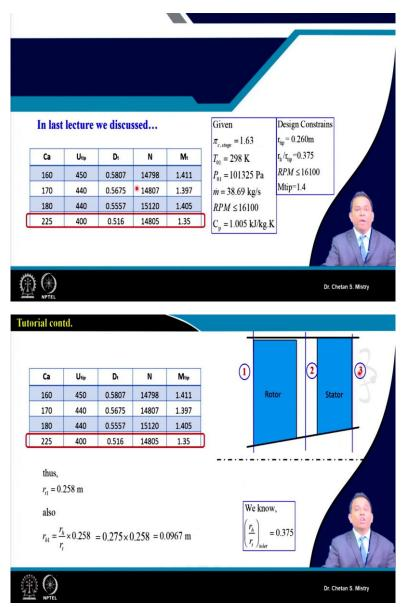
In last lecture, we have discussed about say what data that's what is given to us for the design. It says we are looking for pressure ratio of 1.63, mass flow rate of 38.69 kg/s and we have constraints with say tip diameter, hub to tip radius ratio at the entry that is also fixed, and it says our rotational speed should not exceed by 16,100. In last lecture, we were discussing about
