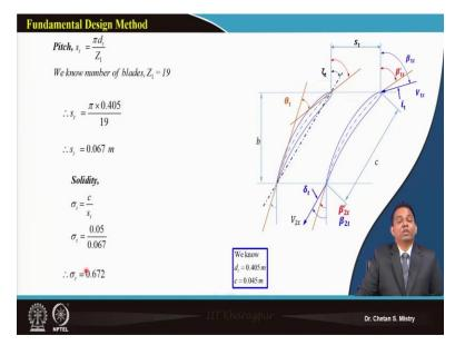
Now, we need to calculate what will be our diffusion factor at the tip station. So, we will be calculating our pitch, we will be calculating our solidity. So, pitch, we are calculating based on  $\frac{\pi d_t}{Z}$ . Here, my number of blades, we are assuming to be 19. So, that's what is giving me my pitch to be 0.067 m. And if you are putting our chord to be 0.045, that's what is giving me say my solidity as 0.67.
