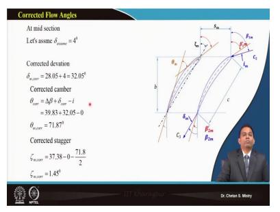
Now for this case, say we have assumed this to be  $4^{\circ}$  and if you do it, say at mid station, we have done calculation for corrected deviation, corrected camber and corrected incidence, okay, or corrected our stagger angle, okay. So, you can say my corrected deviation, corrected camber and connected stagger, we have done calculation.
