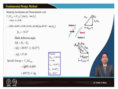
Now, once we have calculated that part, we can do our calculation based on say our comparison, aerodynamic work and thermodynamic work, that's what we are comparing here. And based on this comparison, we can do our calculation for say outlet blade angle, okay, or my air angle, that's what is, or relative flow angle  $\beta_2$ , we are calculating.
