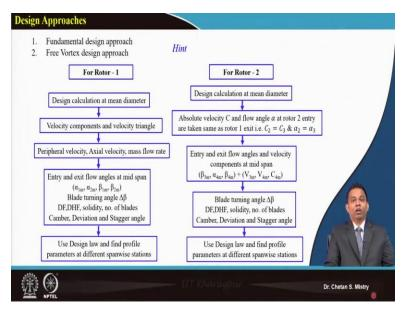
Now, this is what all we have discussed in sense of our hint for solving the problem. So, what we realized? We will be calculating our mean diameter for rotor-1. Then all parameters, that will be calculated at mid station. Based on our design concept or design fundamentals, we will be opting that for say different stations for this blade.
