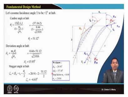
We can do our calculation for say camber angle at the hub, we can do our calculation for the say deviation angle at the hub and we can do our calculation for the say stagger angle at the hub. It says, this is, camber angle is coming 51.12°, my deviation angle, it is coming 15.93, and my stagger angle, that's what is coming -6.65, okay.
