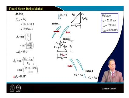
Now, we need to do our calculation since we are having our axial velocity to be different. So, we will do our calculation for different flow angles. So, if we are putting our velocity triangle; so, this is what is a triangle at the hub, we can say our  $C_{w2}$  it is nothing but  $b \cdot r_h$ , this b is our constant, that number we know it is 189.87 and hub radius is 0.1. So, that's what is giving 18.98 m/s.
