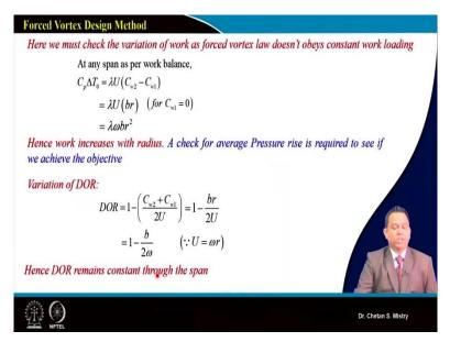
Now, this method we need to check the variation of work as force vortex, that's what is not following constant work loading, okay. So, what we can write down from our fundamental approach, we can say my thermodynamic work and aerodynamic work they both are same. Here in this case, what we know  $C_{w1}$ , that's what is equal to 0 and my  $C_{w2}$ , that's what we are putting say b into r.
