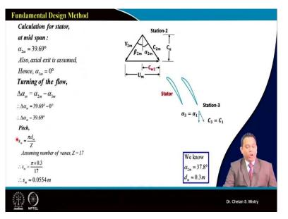
Now, based on that in our next step, that's what will be to design say our stator. And for stator, what we have learned for say stage configuration, rotor-stator combination, we are assuming our absolute velocity coming out from the rotor, that's what will be equal to say our velocity...absolute velocity at the entry of my stator.
