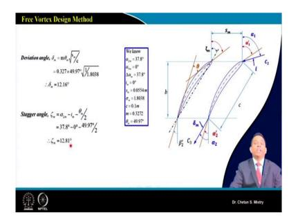
Now, once we have calculated our camber angle, we can do our calculation for the deviation angle. This deviation angle, that's what is a function of my 'm' parameter, my camber angle and solidity. So, based on that we can calculate our deviation angle, that's what is coming  $12.16^{\circ}$ , okay.
