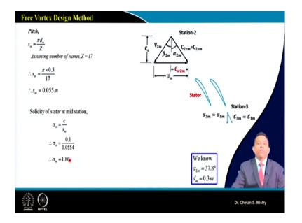
So, in order to do the calculation for say stator, let us see. So, same way what we have done for the rotor, we will be doing our calculation for the stator at the mid station. Here, in this case, what we are assuming, just look at, say, my absolute velocity, that's what is coming out from the rotor, that's what we are assuming same, that's what is entering in my stator. So, you can say,  $C_2$  for rotor and my  $C_2$  for stator, they both are same; this is what is our assumption.
