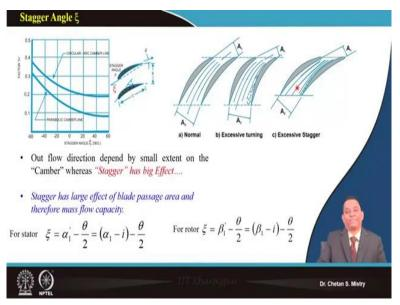
Next, because we have modified now these angles with the metal angles, accordingly we need to do modification in our stagger angle also. So, here if you look at, for stator, that's what is given by this is what is my metal angle  $\alpha'_1 - \frac{\theta}{2}$ , same way for say rotor, we can write down like this.
