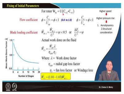
Say, what we know for our rotor, our work done that's what we are defining based on our fundamental Euler's equation. Today let me introduce very important parameter that's what is say flow coefficient. Now, this flow coefficient is nothing but it is a velocity ratio that's what is given by axial velocity divided by peripheral speed at the tip, okay, and it says that need to be less than 1.
