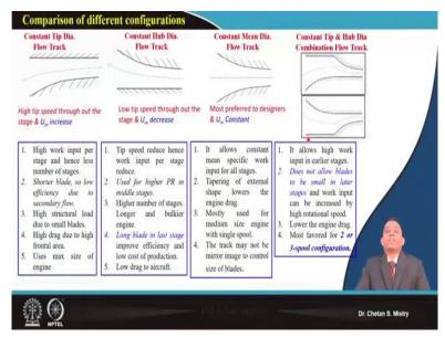
And, if you recall, this is what all we have discussed in sense of different kind of configuration, in sense like constant mean diameter, constant hub diameter, constant tip diameter and combination of flow tracks. Now, suppose we are looking for say number of stages to be reduced, we can say, we will be going with the configuration of constant tip diameter. But at the same time for the later stage, we will be having blade to be very small and that's what will lead to reduce the efficiency.
