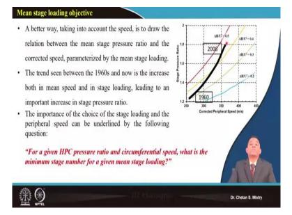
So, here in this case if you look at, this is what is represented my corrected peripheral speed versus my stage pressure ratio and this is what is representing my say stage loading coefficient or mean loading factor, okay. So, this is what is representing the trend from 1960 to 2008; if you look at carefully, its states my mean loading factor or main stage pressure ratio and my peripheral speed they all are increased by some amount, okay, and this is what is a recent trend.
