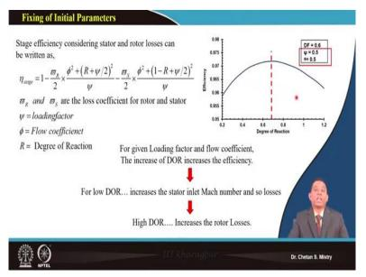
Now, let us take the next case. Say, we are assuming say our loading coefficient and flow coefficient that's what we are fixing with and we are taking the variation of degree of reaction with the efficiency, it says with the degree of reaction to be increased, we will be having efficiency to be rise up to particular extent, okay.
