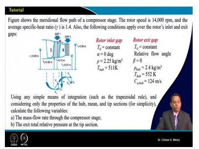
So, take a numerical, say...here it says figure shows meridional flow path of compressor stage. The rotor speed is 14,000 rpm and specific heat ratio is 1.4. The following conditions apply over the rotor inlet and outlet gaps. So, information available at rotor inlet gap is my total temperature is constant. My inlet absolute flow angle is 0. Density is 2.25  $kg/m^3$ . And static temperature at the hub is 511 K.
