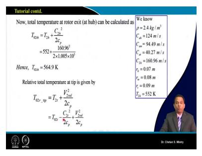
Now, what we are looking for, we need to have temperature to be known in order to calculate our critical velocity ratio, okay. So, at hub, we can straightway write down say,  $T_{02}$  at the hub, that's what is given by my static pressure plus  $C_2$  square by  $2C_p$ , okay.
