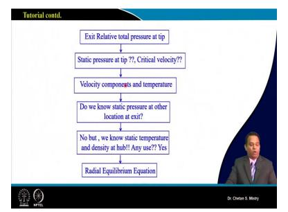
So, let us move with what all we are looking for, it says, we are looking for exit relative total pressure at the tip. And for that we are looking for say static temperature and critical velocity. And in order to do the calculation of this critical velocity, all these steps what we have followed. Now, we are looking for say static pressure, that's what is our target.
