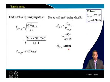
Now, this is what is known to us. So, we can calculate what will be our relative velocity or relative critical tip velocity, that's what we know that is given by  $2\gamma$  RT<sub>02</sub> at the tip, that's what is a relative temperature by  $\gamma + 1$ , that's what we are calculating as say 431.26 *m/s*, okay.
