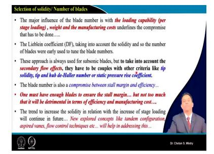
Here, if we consider say number of blades, then we need to realize what kind of loading we are looking for. That means per stage loading what we are expecting. Second parameter, that's what is coming into the picture is a weight of that rotor and because of the weight of that rotor, the weight of whole engine. Then we need to check for say manufacturing cost and we need to compromise in sense of all these parameters.
