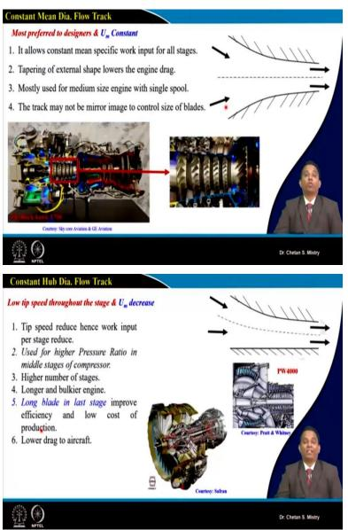
Now, this is what is a configuration in which I am having my mean diameter that's what is constant; you can see, this mean diameter it is constant, okay. And this is what people used to say it is a most preferred design to add up or to go with a constant mean diameter kind of configuration, okay. So, it says it allows constant mean specific work input for all the stages; that's what is a big benefit, okay. If you consider we are having tapering of this external surface; that's what is going
