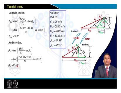
In line to that, we can calculate what is our angle at the midsection and that's what is coming  $10.2^{\circ}$ . Similarly, at the tip station also, we can calculate our angle and that angle is coming  $13.48^{\circ}$ .
