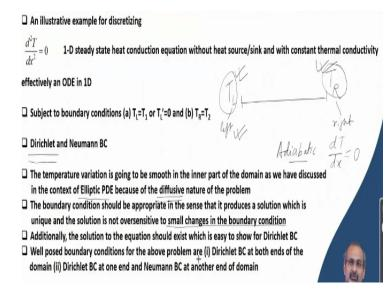
We will now try to do an illustrative example. We are going to discretize the one-dimensional steady state heat conduction equation without any heat sources or sinks and with constant thermal conductivity. We have come across this equation earlier when we talked about the Laplace equation and Laplace equation in general could be in multi-dimensions, but here we have reduced it to one dimension.
