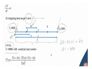
Let us look at the domain that we have set for ourselves. So, here is a one-dimensional domain of length L which we have set equal to 0.1 meter and we have a left end temperature equal to 600 K (Kelvin) and the right end temperature of 200 K and we want to find out by using a finite difference approximation that how temperature could vary in the intermediate domain, that means this region, just leaving apart the boundary conditions.
