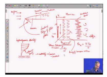
Let us try to make a small sketch of a flat plate over which a uniform flow is impinging. So, this is the leading edge of the flat plate. You know that there is a formation of a boundary layer. Initially, it remains laminar then there is a region where it starts developing disturbances and then there is a region where it has become completely turbulent and therefore eddying structures fill the flow.
