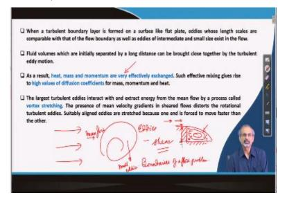
When a turbulent boundary layer is formed on a certain surface say like a flat plate on an airfoil. Eddies of different length scales can coexist large small intermediate that we already talked about. And fluid volumes moving around on that surface are initially separated by long distances. But at some point of time can be brought together because there is a lot of fluctuations in the velocity components which can augment the transport, transport of heat mass momentum everything gets augmented.
