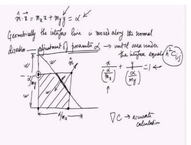
And we are trying to figure out how to reach there. So, we are saying that it can be reached by adjusting this parameter alpha. And geometrically how it is done can be shown through a small diagram. Let us say, we have a certain cell here. And let us say the interface lies somewhere here. And this is the marker filled region. So, the straight line is the one which we have indicated here.
