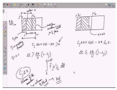
Let us make a small diagram here or rather a pair of diagrams, so, that we can see the two scenarios. So, these are the two cells. Let us say, this is the j cell; this is the j + 1 cell. So, this is j plus half interface; this is j minus half interface. And let us assume that at this point of time the C j has been defined this way that C j times delta x shows the dashed region. Now, remember that C j is essentially acting like a weighting function.
