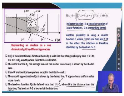
So, here we are talking about an interface region. You can understand this is the interface region where the Heaviside function has dropped down sharply. And you can see that because color function is essentially an integrated effect of the Heaviside function how it is defined within a certain cell. Therefore, the color function occupies this gray region as though the cell is getting filled up from bottom up.
