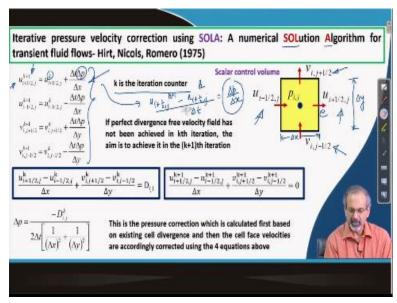
And this is one of the most popular approaches in solving incompressible Navier Stokes equations. We are also proposing another very elegant iterative pressure velocity correction using a scheme which is called as the SOLA scheme. So, the full form of this scheme is a numerical solution algorithm for transient fluid flows, which was proposed by a few scientists headed by Heart.
