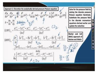
Another approach could be that we use the discrete analytically derived pressure Poisson equations. So, earlier lectures have shown how to obtain the pressure Poisson equation analytical by taking derivatives of the moment of the equation suitably summing them up and then we come to the pressure Poisson equation. So, we have actually picked up that form and we are trying to demonstrate that even from that form, you can possibly solve pressure.
