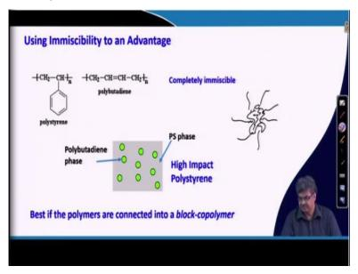
Now we can use this immiscibility to our advantages, for example polystyrene is a brittle polymer. Now to improve the impact behavior or ductility of polystyrene, this rubber polybutadiene rubber is added. Now if they were completely miscible then we would have a single phase and the impact property of polystyrene would have increases marginally because of presence of polybutadiene.
