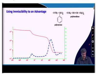
And if we do a DMA of this polystyrene polybutadiene sample, we can see that this is a T g corresponds to the polybutadiene phase and this is T g corresponds to polystyrene phase and this is tan delta. So, you can see there is a maximum here corresponds to the T g of polybutadiene and there is a maxima around little over 100 degree which corresponds to the maxima corresponds to the T g of polystyrene molecule.
