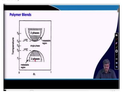
And this is a possible phase diagram, not necessarily each polymer pier will have all these LCST and different region. This is the total possible scenario which captured in this phase diagram. And this value corresponds to lower critical solution temperatures, which means below this
