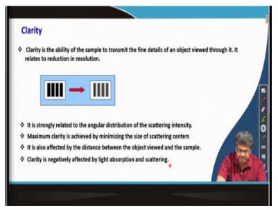
We often use the term clarity, what is the actual meaning of clarity? Clarity is the ability of a sample to transmit the fine details of an object viewed through it. So, if you are being through a polymer glass then this ability to transmit the fine details of an object is related to the clarity of the polymer sample through which we are viewing and it relates to the reduction in resolution. So, you can see this graph to understand this, this sketch to understand this.
