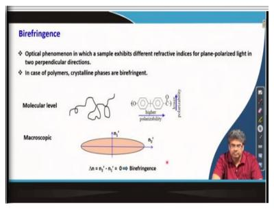
This also another term related to optical properties is birefringence. This is related to the optical phenomena in which a sample exhibits different refractive index for plane polarized light into perpendicular direction. If we use 2 differently plane polarized light and if it is show different
