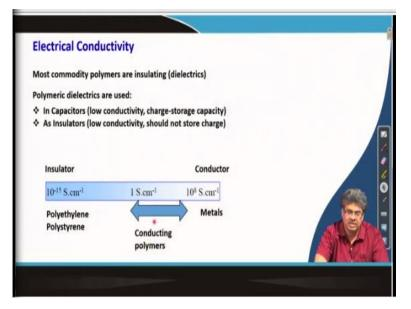
We will move to next property electrical property and again I will just briefly touch these properties. Most polymers or commodity polymers are insulating dielectric and this is very advantageous because polymers are used for many applications as electrical, electric insulators. And as a result polymer dielectrics are used in capacitors, low conductivity, charge storage device and as an insulator which require low conductivity and should not store charges.
