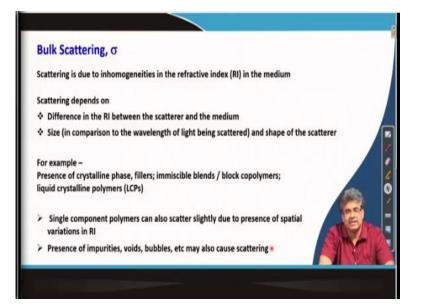
Let us talk about bulk scattering, now bulk scattering is due to in homogeneities in the refractive index of the medium. If the medium has more than one component and their refractive index values are different then the sample will actually scatter light. And this scattering depends on the difference in the refractive index between the scatter and the medium. And of course on the size in comparison to the wavelength of the light being scattered and the shape of the scatter.
