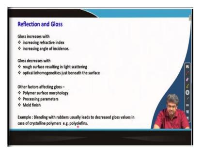
Gloss increases with increasing refractive index, increasing angle of incidence and gloss decreases with rough surface resulting in light scattering, optical inhomogeneities just beneath the surface. And other factors which affects gloss are polymer surface morphology, processing parameters, mold finish. For example blending with rubbers usually lead to decrease in gloss value in case of crystalline polymers like polyethylene.
