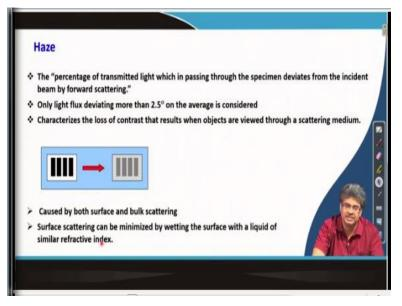
Now we talked about haze, what is haze? Haze is a percentage of transmitted light which is passing through the specimen deviates from the incident beam by forward scattering, which means only light flux deviating more than 2.5 degree on average is considered. It characterizes the loss of contrast that results in objects are viewed through a scattering medium.
