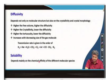
We talk about diffusivity, diffusivity depends not only on the molecular structure but also on the crystallinity and crystal morphology of the polymer sample. Higher the free volume of obviously the space is higher, so how higher will be the diffusivity. Higher is the crystallinity lower would be diffusivity as one can easily understand. And if the path, diffusion path is torturers, so if we add some clay materials in between.
