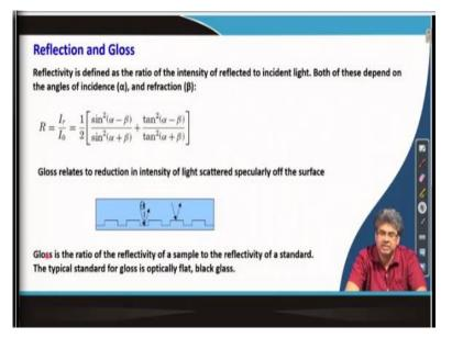
We will also talk about the terms reflection and gloss, reflectivity is defined as the ratio of intensity of the reflected to the incident light. Both of these depends on the angle of incidence and refraction alpha and beta. And this is related to the intensity of the reflected light to the intensity of the incident light and this is given by this expression where angle of incidence is alpha and refraction, angle of refraction is beta.
