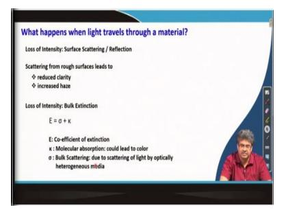
Now before we discuss the optical properties, we need to find out or we need to understand what happens when light travels through a material or when light interact with material. Invariably there will be loss of intensity due to surface scattering or reflection and due to the bulk scattering or extinction. So, let us talk about the surface scattering, the surface scattering happens because of the rough surface and these actually reduce clarity and also increase haze in the polymer sample.
