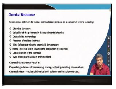
Next we will move to the next property chemical resistance. Now chemical resistance is a resistance of polymers to various chemicals. And which depends on a number of criteria which includes chemical structure. Solubility of the polymer in the experimental chemical obviously if the polymer is more soluble the chemical will have chance to degrade or interact with the polymer in a more than if it was not soluble.
