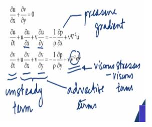
You can see the two-dimensional incompressible Navier Stokes equations in the screen. It is comprised of mass conservation and momentum conservation equations. So, the mass conservation equation is more often called as a continuity equation because it is two-dimensional Navier Stokes equation. So, you have 2 components of velocity respectively u and v and both of the velocity components are functions of x and y.
