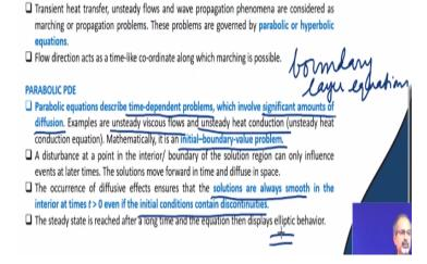
In marching problems, we can be solving transient heat transfer or we may be solving unsteady flows or wave propagation phenomena, where we can see the solution changing with time. These problems are governed by parabolic or hyperbolic equations and in these problems sometimes a particular flow direction can also act as a time-like coordinate along which we can march the solution. So, this is what we see in say boundary layer equations.
