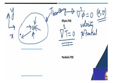
Here we have a curve drawn in two-dimensional space and we are trying to understand how an elliptic partial differential equation would behave when we are solving it in a domain like this. So, in this domain if you look at a certain point you will find that information is propagating into that point from all directions and also information from this point can affect other points in its vicinity.
