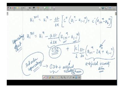
As we do this we can represent the first order upwind scheme in a more general form where you can cater to both positive as well as negative wave speeds. So, this is how one write it and if you substitute the values of C+ and C- and do a little bit of arrangement, you will be in a position to show it this way. So, this is the final form as you can understand that this contribution comes from a central differencing.
