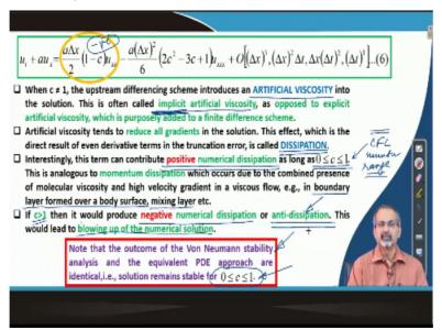
Now, whenever c is not equal to 1, what this term is going to do is. It is going to introduce a very important property which is called as artificial viscosity. That means, it is going to play the role similar to molecular viscosity, what you see in viscous simulations of the problem through Navier Stokes equations. So, this comes automatically by virtue of the numerical scheme that you were using.
