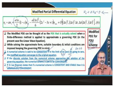
In the previous lecture, we had discussed about the modified partial differential equation. So, we are revisiting that equation here in the starting slide. So, we remember that we did it for the first order upwind scheme for discretizing the linear wave equation and we could identify that there are error terms in the truncation error and incidentally, the leading error term happens to be a second order derivative in space associated with a coefficient.
