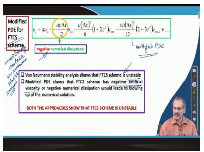
If we quickly recall about the forward time central space scheme for discretizing linear wave equation, we remember that it did not work because it was unconditionally unstable. This, we have shown through the Von Neumann stability analysis. So, though it is not an useful scheme, we would like to revisit it once more just to see that how does the modified partial differential equation form of the FTCS scheme look like?
