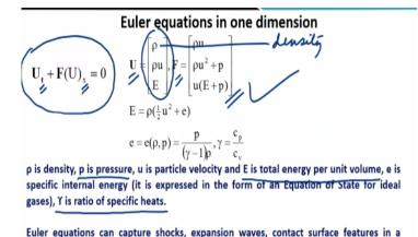
Compressible medium. Here Euler equations is expressed in flux vector form, where U is the column vector of conserved variables and F(U) is flux vector.
